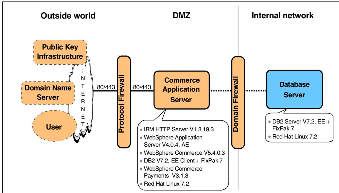
Figure 4-1 Product mapping for the two-tier remote DB2 server runtime for Linux
